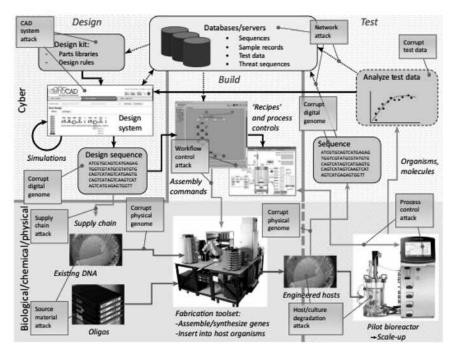
Figure 4 Cyber-Physical Bio-manufacturing process
