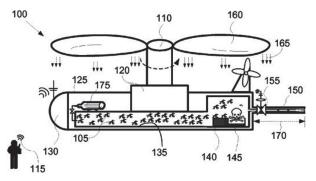
Figure I Toxic Mosquito Aerial Release System - Patent US-8967029-BI
