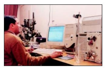
Analysis of High Explosive substance by High Pressure Liquid Chromatozraphy system in CFSL (CBI), New Delhi
